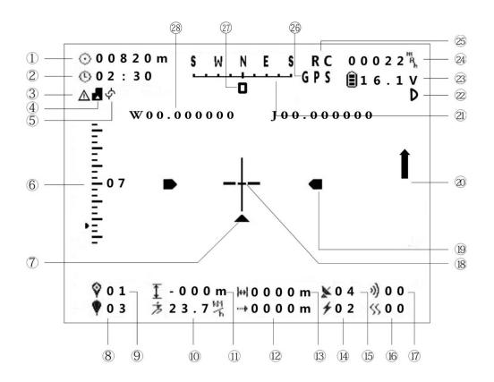
① Radius of target area (Unit: M,for ordinary edition),angle offset of camera holder (Unit: degree,for gemini edition).
